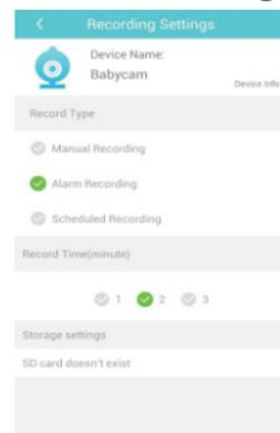
**Manual Recording:**24 hour recording continuously. Not recommended because it occupies too much TF card storage.
